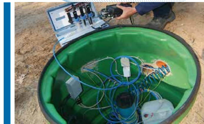
Gas storage technology BIOXWAND, Pat. DE102004001802 – Clean gases or gas mixtures are stored in the pore space of the soil matrix, forming permeable gaseous reactor curtains.
