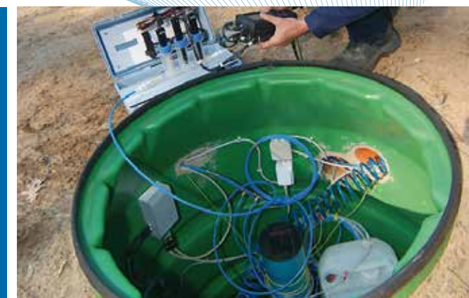
Gas storage technology BIOXWAND, Pat. DE102004001802 – Clean gases or gas mixtures are stored in the pore space of the soil matrix, forming permeable gaseous reactor curtains.
